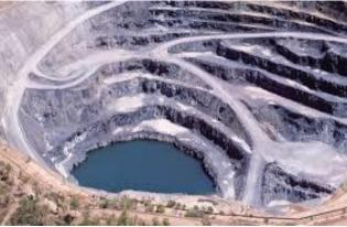
Example of an open pit with effective. Groundwater control. The pit floor is far below the elevation of the predevelopment groundwater table.
